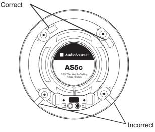
With the grill removed, place the speaker in the ceiling opening. Make sure that the speaker wire is not hanging against the speaker where it can vibrate and rattle as the speaker reproduces your audio program.
